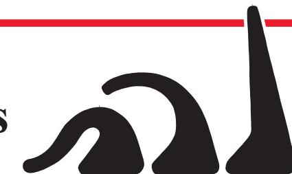
Pyrometric cones have been used to monitor ceramic firings for more than 100 years. They are useful in determining when a firing is complete, if the kiln provided enough heat, if there was a temperature difference in the kiln or if a problem occurred during the firing.
